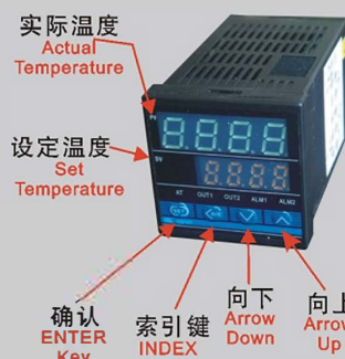
智能数显温控表、温控±1℃ Intelligent digital display temperature control meter, temperature 1℃±
